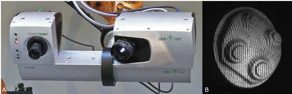
Figure 11. Fringe projector (A) and fringe projected on a complex surface (B)
