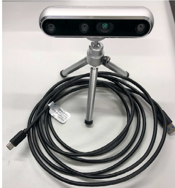
Figure 32. Intel real sense camera and usb c connector
