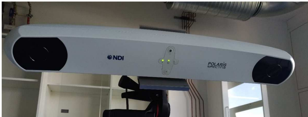
Figure 31. Position sensor, showing the steady green LEDs on (center of the device) for correct system operation
