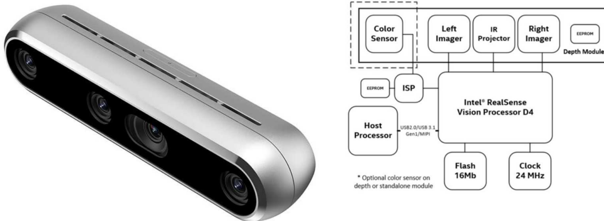
Figure 29. Intel® RealSense™ D455 depth camera (left panel) and camera system block diagram (right panel)
