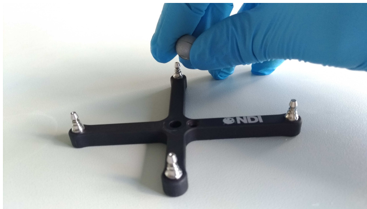
Figure 20. Handling of passive markers
