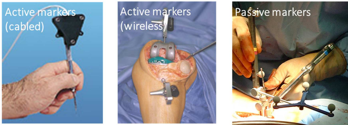
Figure 1. Markers utilized by IR optical tracking systems.
