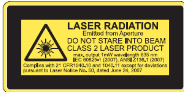
Figure 15. Laser radiation warning on the Hybrid Polaris Spectra
