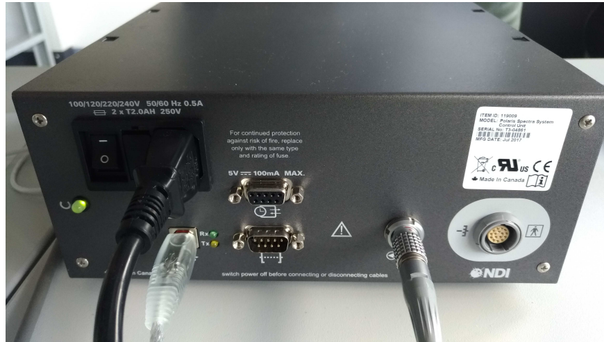
Figure 30. Rear panel of the SCU, with the power button on the left side of the power cable
