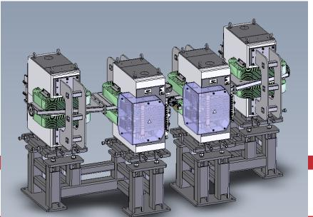
30-20 mm collimator upstream and downstream the chicane (200 mm far from dipoles)
