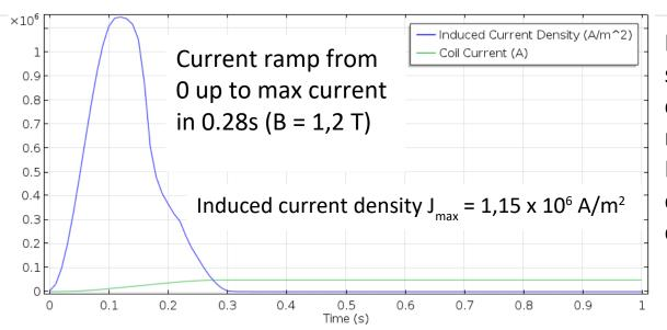
If the current is changed each second (each laser shot) the system could be used as an active energy modulator system Induced sextupole due to the eddy current on the vacuum chamber can be neglected after 0.31s
