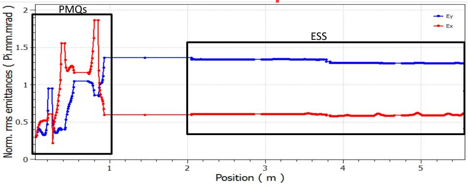
Emittance growth limited to the PMQs system and due to filamentations in the PMQs
