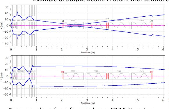
Beam envelope for reference beam 60 MeV protons and phase space plot at the ESS output
