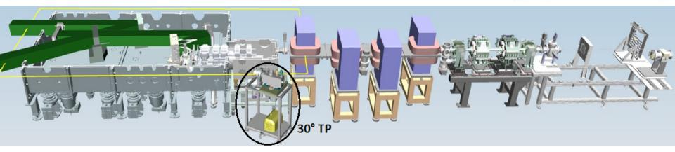
No space for an on-axis spectromete, but Dipole 1 in the chicane is independently calibrated This Dipole can be used a magnetic deflector for a Thomson Parabola and it can resolve protons up to 300 MeV and carbons up to 75 AMeV
