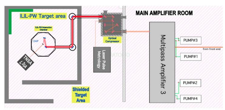
Figure 1: Lay-out of ILIL-PW system comprising the main multi-pass amplifier, compressor, and target area [2].
